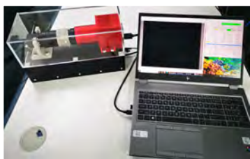
Star tracker's Host computer +Image acquisition software
