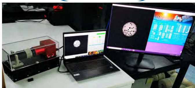
Star TRACKER+Dynamic star simulator +Image acquisition system
