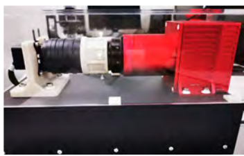
Star TRACKER+Dynamic star simulator +Image acquisition system
